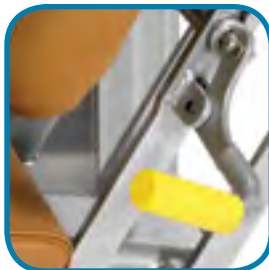
Seat back adjustment lever
