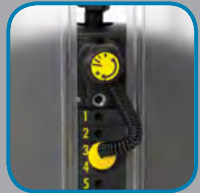
Twist select low increment weights
