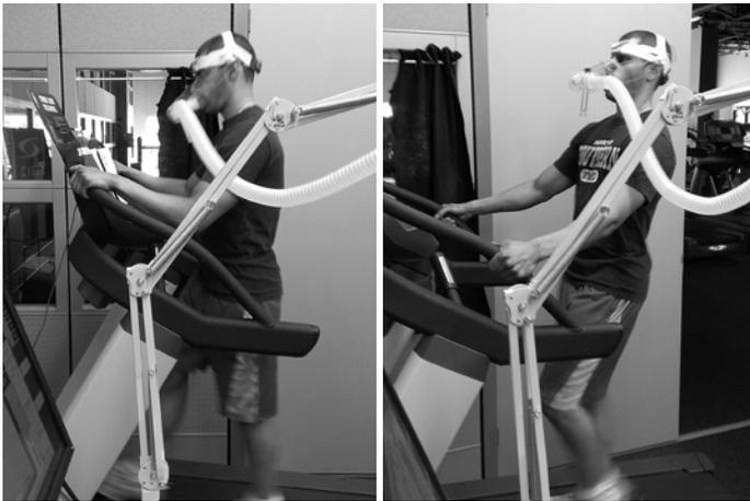
Figure 1. Handrails used in the present study. Subjects were instructed to either walk unsupported (not holding onto anything) or to grasp at a self-selected location and to use the handrails to either 'lean back' (right) or 'remain upright' (left) during experimental trials.
